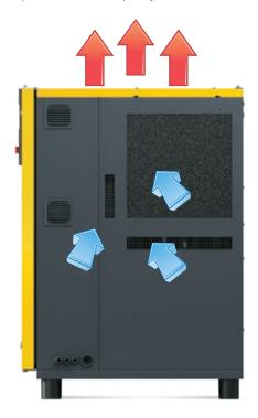
To increase reliability and reduce maintenance costs, the coolers are conveniently located on the outside of the unit, where dust and dirt build-up are easily seen and can be removed without dismantling the cooler. Top exhaust allows for easy heat recovery and reduces the system footprint.
